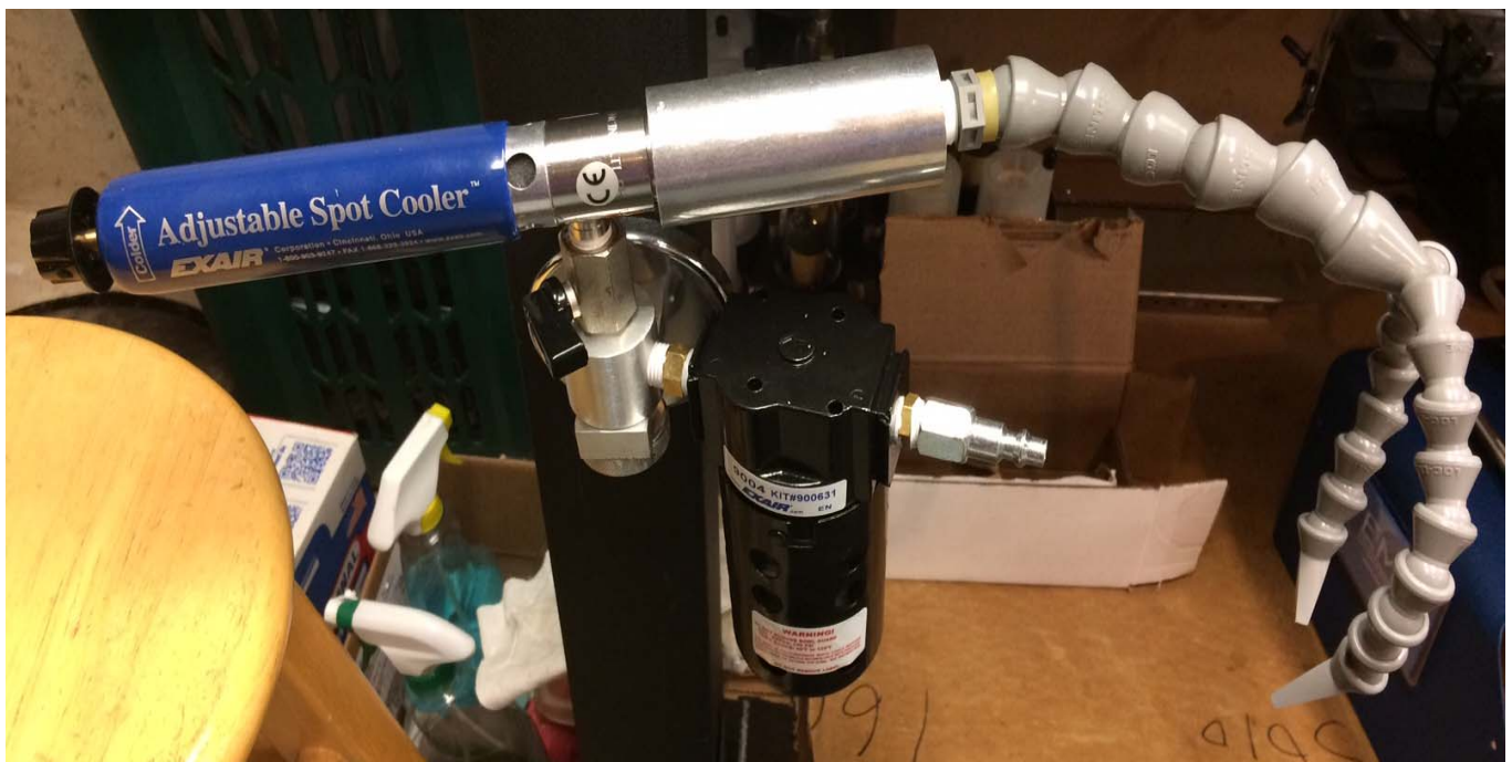
Spot Cooler with compressed air from "Exair"
